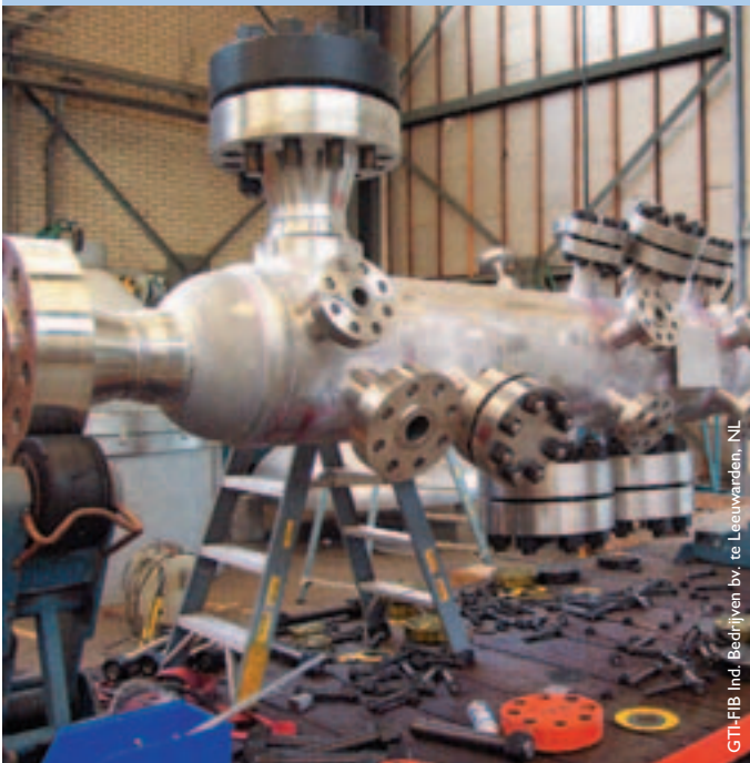
化工设备：UNS S 31803/1.4462，壁厚30~40mm 采用伯乐CN 22/9N-FD焊接
